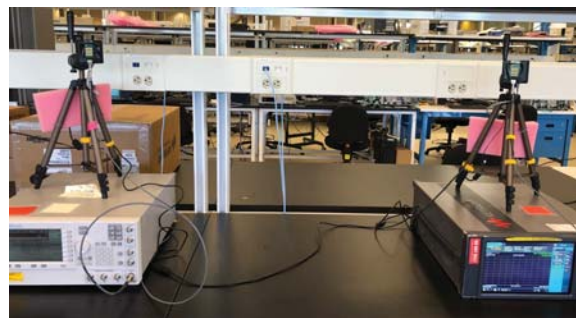
Fig. 7. Test setup using 4 \times 4 UPAs both at the Tx and the Rx side, signal generator, and vector signal analyzer.
